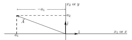
Each physical vector is identified with a string of three numbers,  $(x_1, x_2, x_3)$  or (x, y, z). For example, the y component  $a_2$  of the vector  $\vec{A}$  is its projection onto the y axis, measured as a multiple of the unit vector or basis vector  $\hat{j}$  along that axis.
