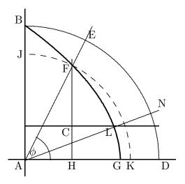
The defining property of the curve can be restated this way: The ratio of the lengths AB and FH equals the ratio of the arcs BED and ED — which is the same as the ratio of the angles BAD (90°) and EAD. In modern notation, if  $\rho$  is the length AF and the circle has radius a, then
